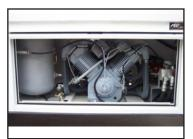
H150 air compressor with PTO/hydraulic drive. 127 CFM with a 23 or 38 gal. tank.
